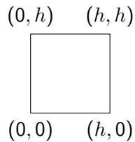
one can construct a unique ansatz function from the four function values at the edges.
